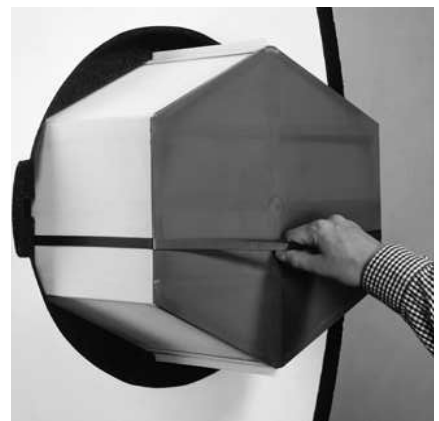
Removing the Heat Exchanger
