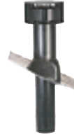
Roof Cowl Ref. 91277AA • Outlet cowl complete with flashing • For roof pitch 25-45° • Insulated, self extinguishing EPS • Colour: black • 160mm diameter (135mm not including foam lining)
